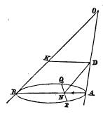
circular section through B, the line of intersection PQ will be parallel to BT, and therefore perpendicular to the diameter BA through B.
